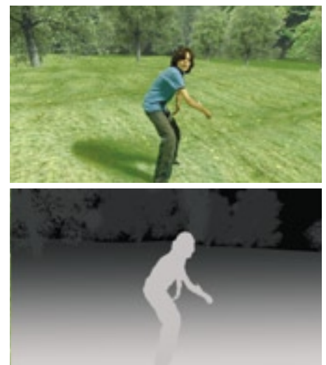
Figure 2: The 2D-plus-depth format is used as the 3D video format in our 3D display systems. (Top) A conventional 2D image providing 2D compatibility and 3D texture information. (Bottom) Depth map providing 3D geometry information by depth-per-pixel.
